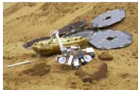
Beagle 2 is it would look after landing on Mars. Image courtesy of Beagle 2.
